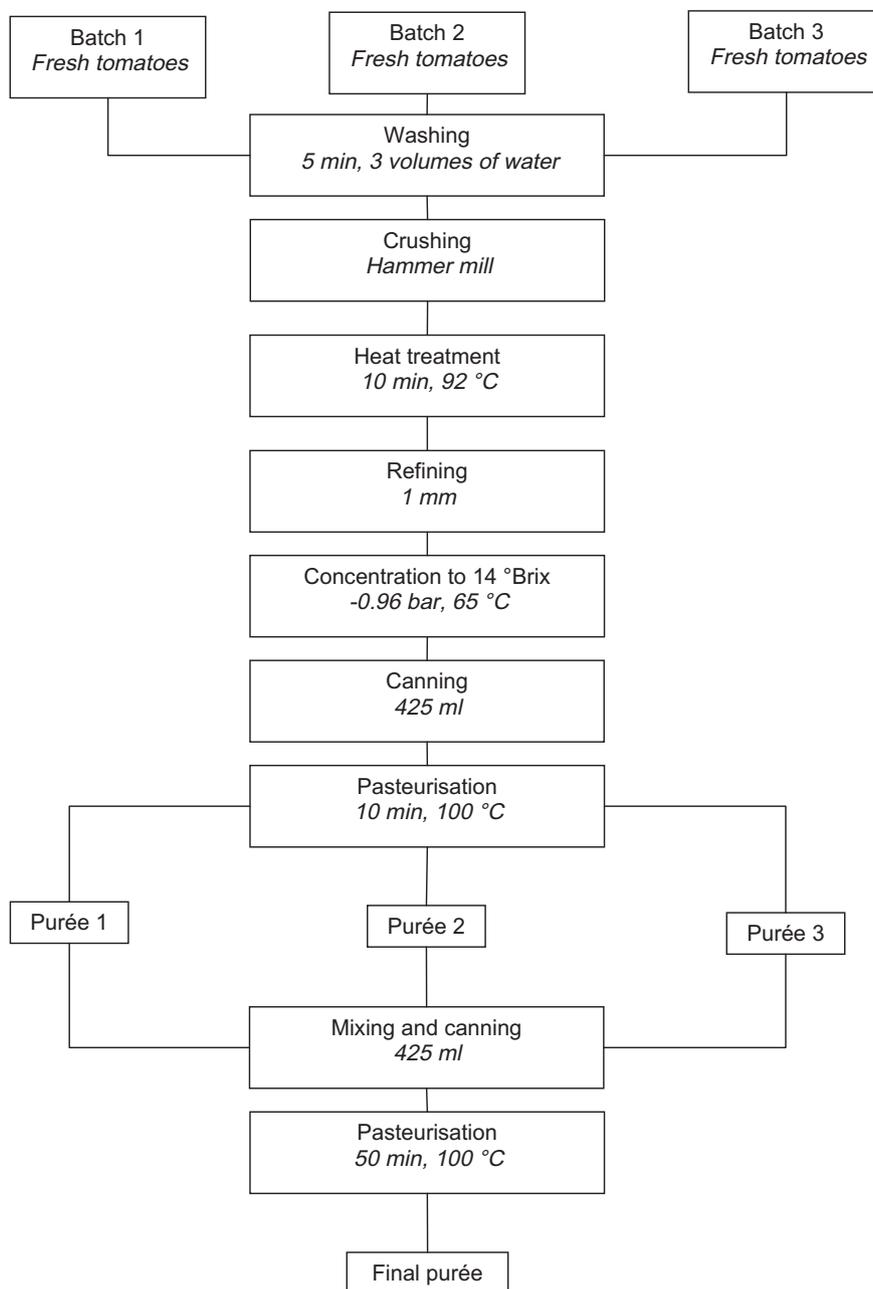
Fig. 1. Description of the process used to obtain red and yellow tomato purées.
